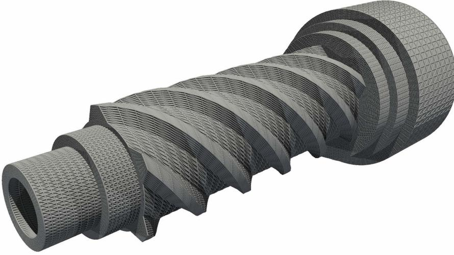
Figure 7.4: As real-world test case, we solve a boundary integral equation on a complex gearwheel geometry. The overlying mesh corresponds to a discretization with  $N = 296960$  boundary elements.
